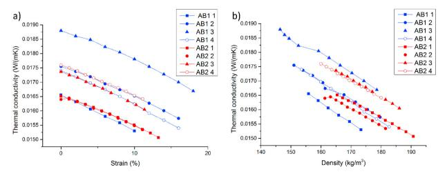
Figure 1. Apparent thermal conductivity of aerogel insulation blankets AB1 (4 specimens) and AB2 (4 specimens) as a function of (a) percentage strain and (b) density.
