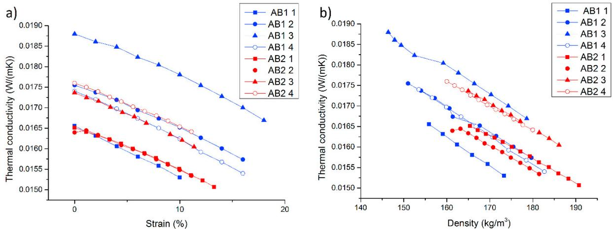
Figure 1. Apparent thermal conductivity of aerogel insulation blankets AB1 (4 specimens) and AB2 (4 specimens) as a function of (a) percentage strain and (b) density.
