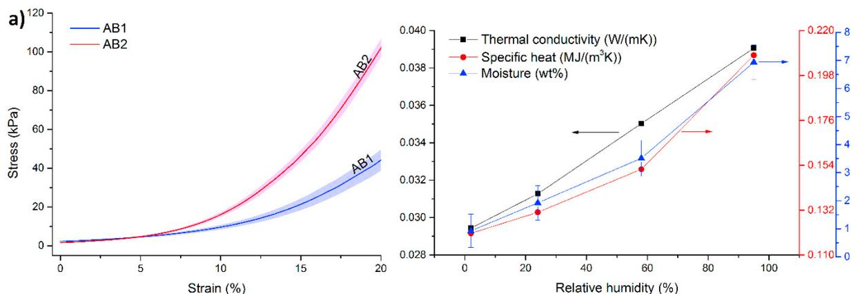
Figure 2. (a) Stress-strain correlation for aerogel insulation blankets AB1 and AB2. The solid lines represent the average of 5 measurements, and standard error of the mean is indicated by the shaded areas. (b) Correlation of thermal conductivity, specific heat and moisture content for aerogel insulation blanket AB2. The standard error of the mean for moisture content is indicated with error bars.
