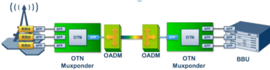
Figure 2.7: Optical transport network[PMC15]
