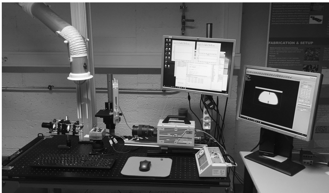
Figure 3.2 - Sessile drop experimental apparatus
