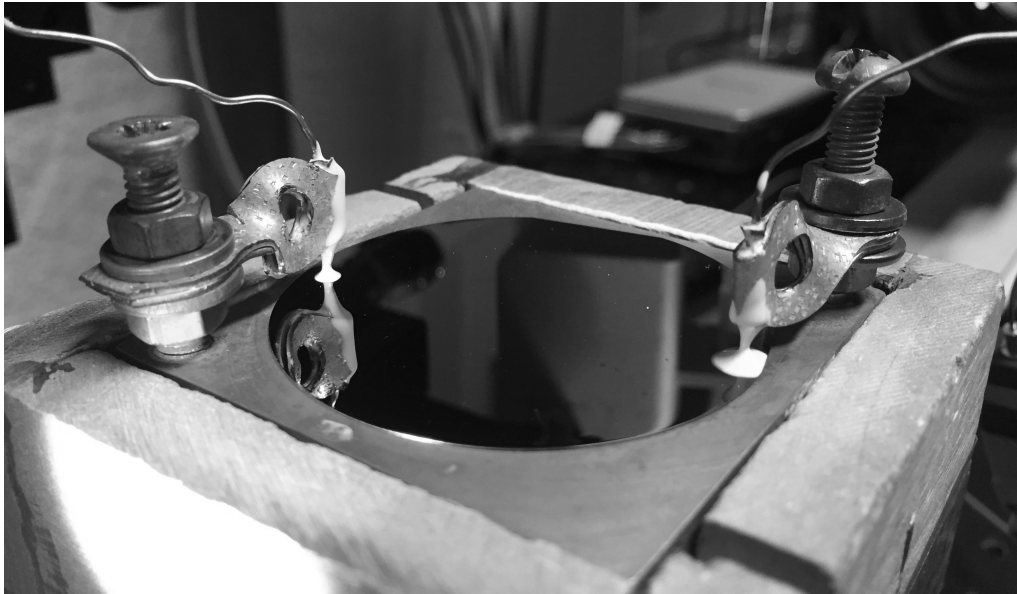
Figure 3.13 – Surface thermocouples designed mechanism
