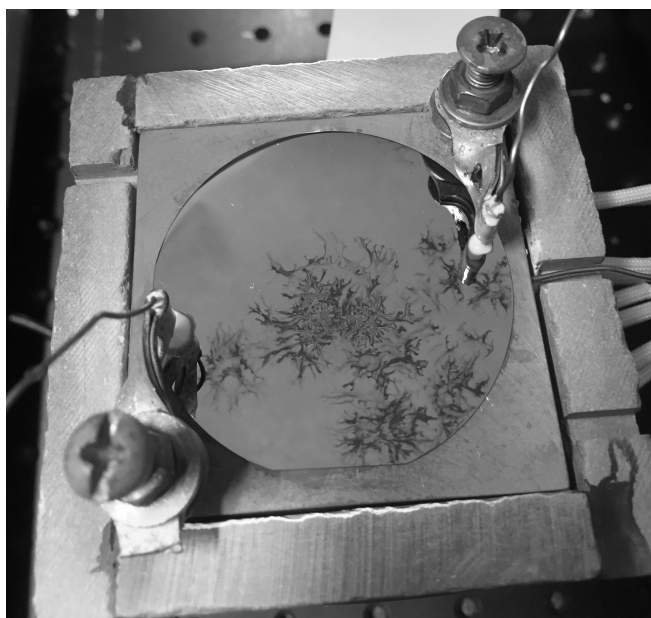
Figure 4.30 – HFE 7000 droplet spot on the plain silicon surface
