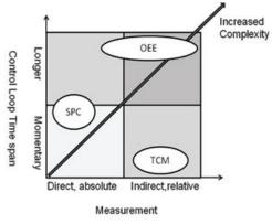
Fig. 1. Classification of Process Monitoring and Control systems
