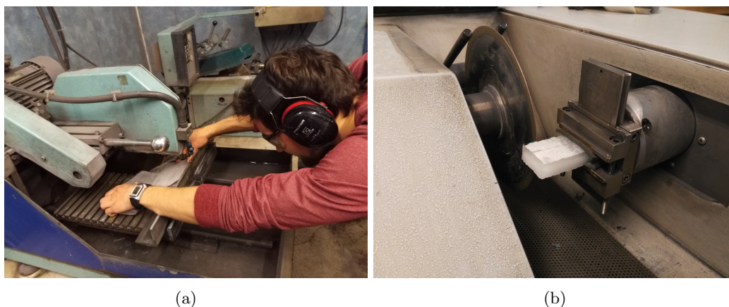
Figure 15: Pictures of the coarse diamond blade saw (a) and the Accutom high precision saw (b).
