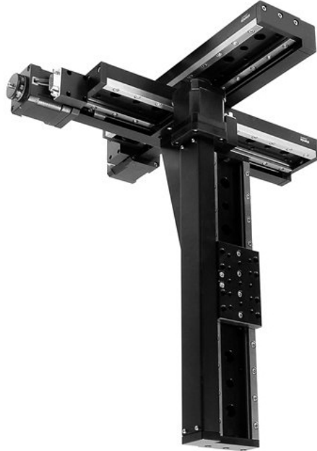
Figure 2.12: XYZ Linear stage combination setup an axes direction as described above adapted from [33].
