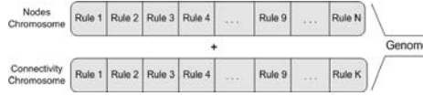
Fig. 4. This is how the genome looks like with the genome split into two ( chromosomes ). The first chromosome is responsible for generating the cells/nodes whereas the second chromosome is responsible for generating the connectivity of the network
