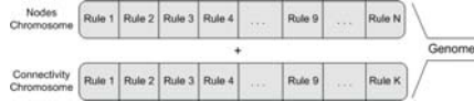
Figure 1: This is how the genome looks like with the genome split into two ( chromosomes ). The first chromosome is responsible for generating the cells/nodes whereas the second chromosome is responsible for generating the connectivity of the network.
