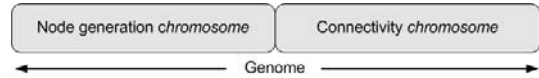
Fig. 5. The common genome with the two chromosomes. The first chromosome maps the cell/nodes of the target architecture. The second chromosome maps the connectivity.
