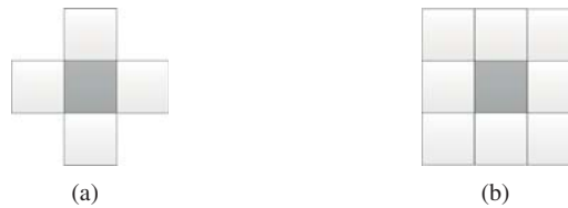
Figure 2.6: Neighborhood structures for two dimensional cellular automata: (a) von Neumann neighborhood, (b) Moore neighborhood.
