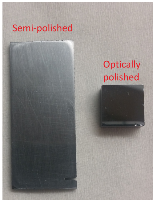
Figure 5.4: The two (LEFT) Semi-polished and (RIGHT) Optically polished Silicon samples.
