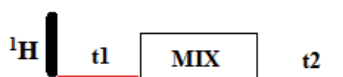
Figure III.1.3.1. Schema illustrating the two time periods giving in 2D spectrum. t_2 is the observed signal, while t_1 is the incremented indirect dimension. MIX is the sequence used to ensure that the signal is transferred between spins. Horizontal black bar is the preparation pulse; the red bar illustrates the signal in different evolution dimensions.
