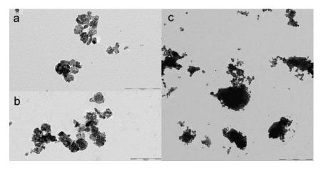
Figure 1: TEM images of  $TiO_2NP$  a) in water (stock solution; scale bar 200 nm); b) Single particles in seawater (scale bar 200 nm); c) Large agglomerates in seawater (scale bar 1µm).
