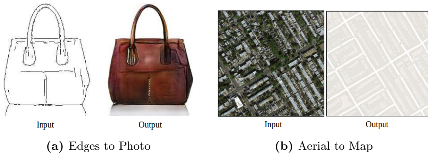
Figure 2.15: Isola et al. [2016] introduced the concept of image-to-image translation using GAN. Due to the multiple correct outputs for each input a generative model is suitable for training the model. Figure 2.15a shows examples of inference when the model is trained to colorize and fill out an outline of an object, while Figure 2.15b shows a model trained to convert from aerial photos to maps. Taken with permission from [Isola et al., 2016].
