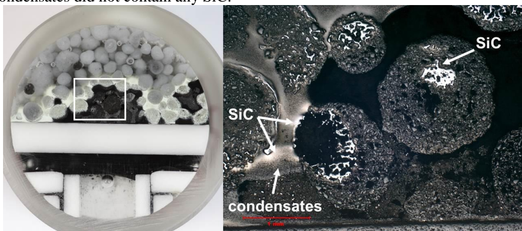
Figure 6. Sample from experiment no. 9. From the right light microscope images of the pellets, condensates and SiC.
