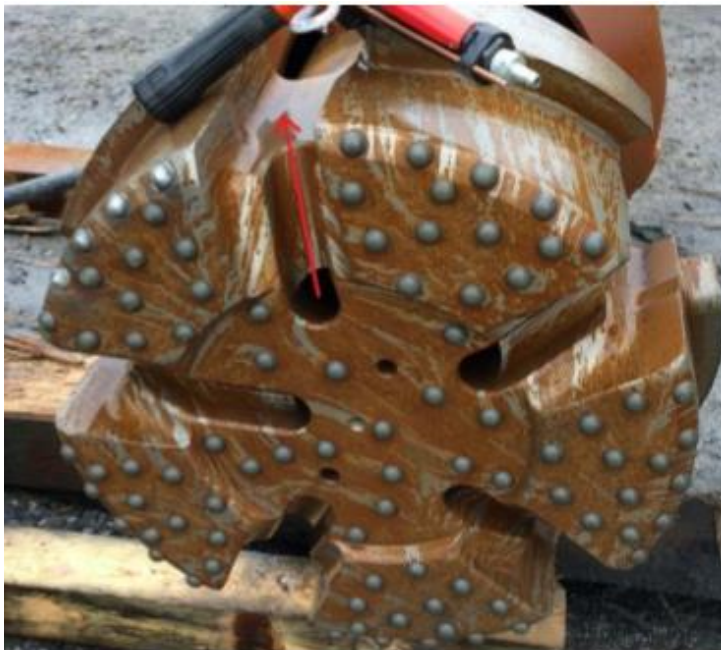
Figure 3-3: Picture of the pilot bit with flushing and return channels (Haugen, Ahmed et al. 2015).
