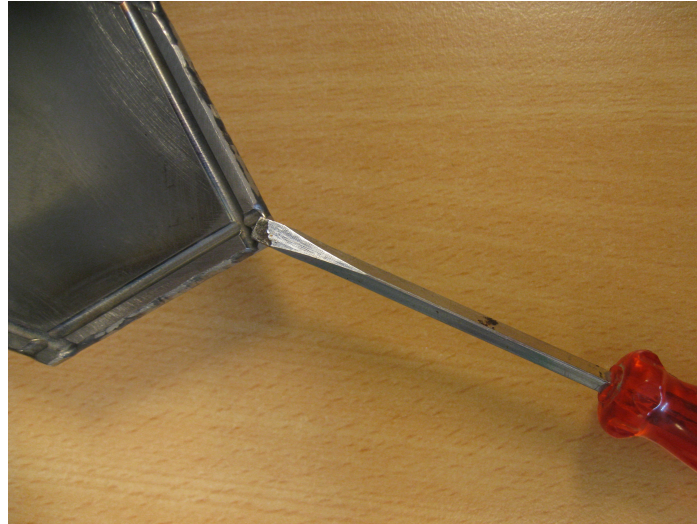
Figure 6.2: Close-up of the test setup for quantifying the effect of elastic bending.
