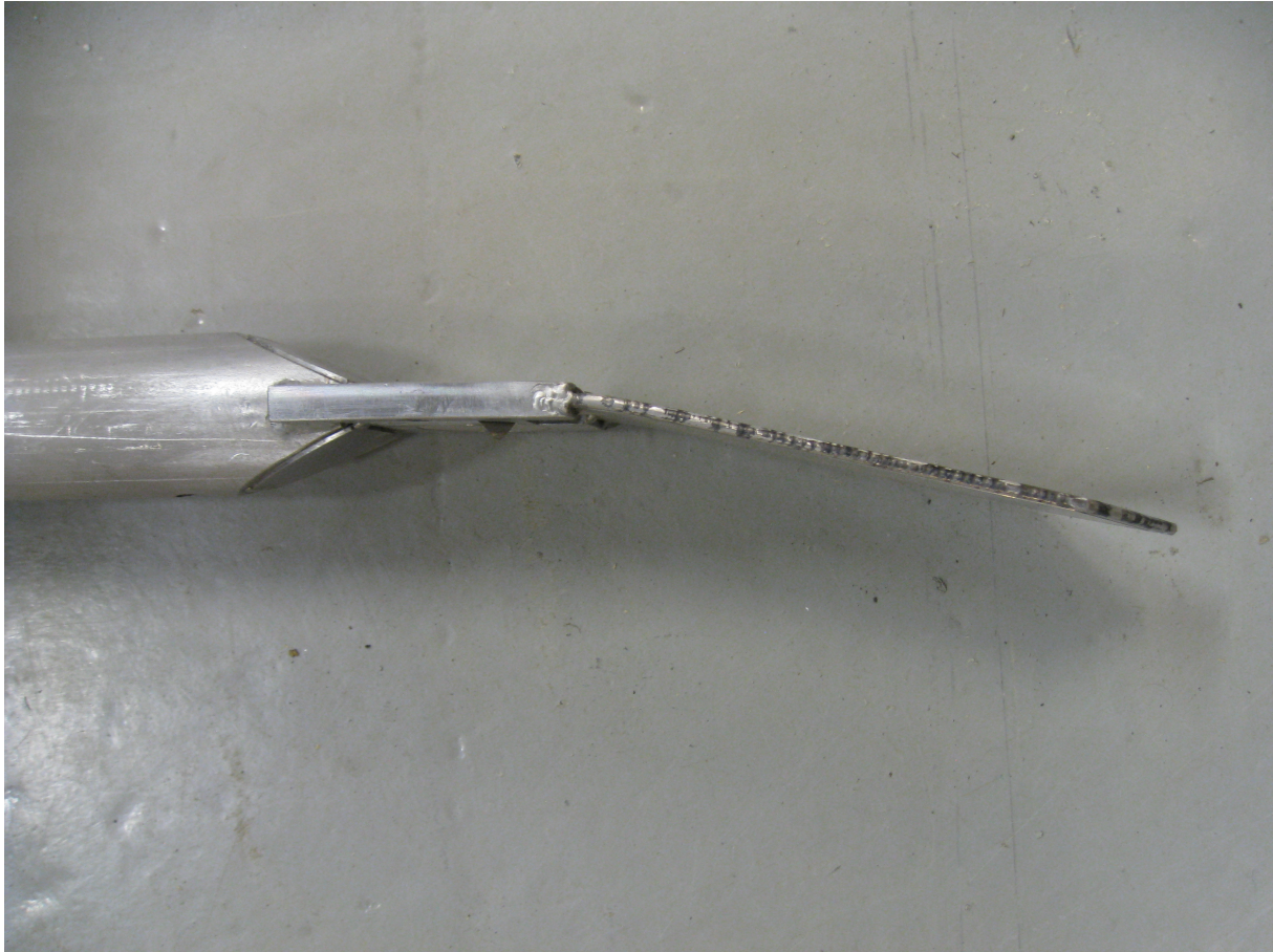
Figure 3.2: Cell damaged during penetration to 6 m. Earth pressure sensor EE24694.
