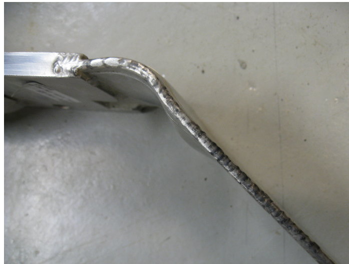
Figure 6.3: Permanent misalignment of the earth pressure membranes due to bending.
