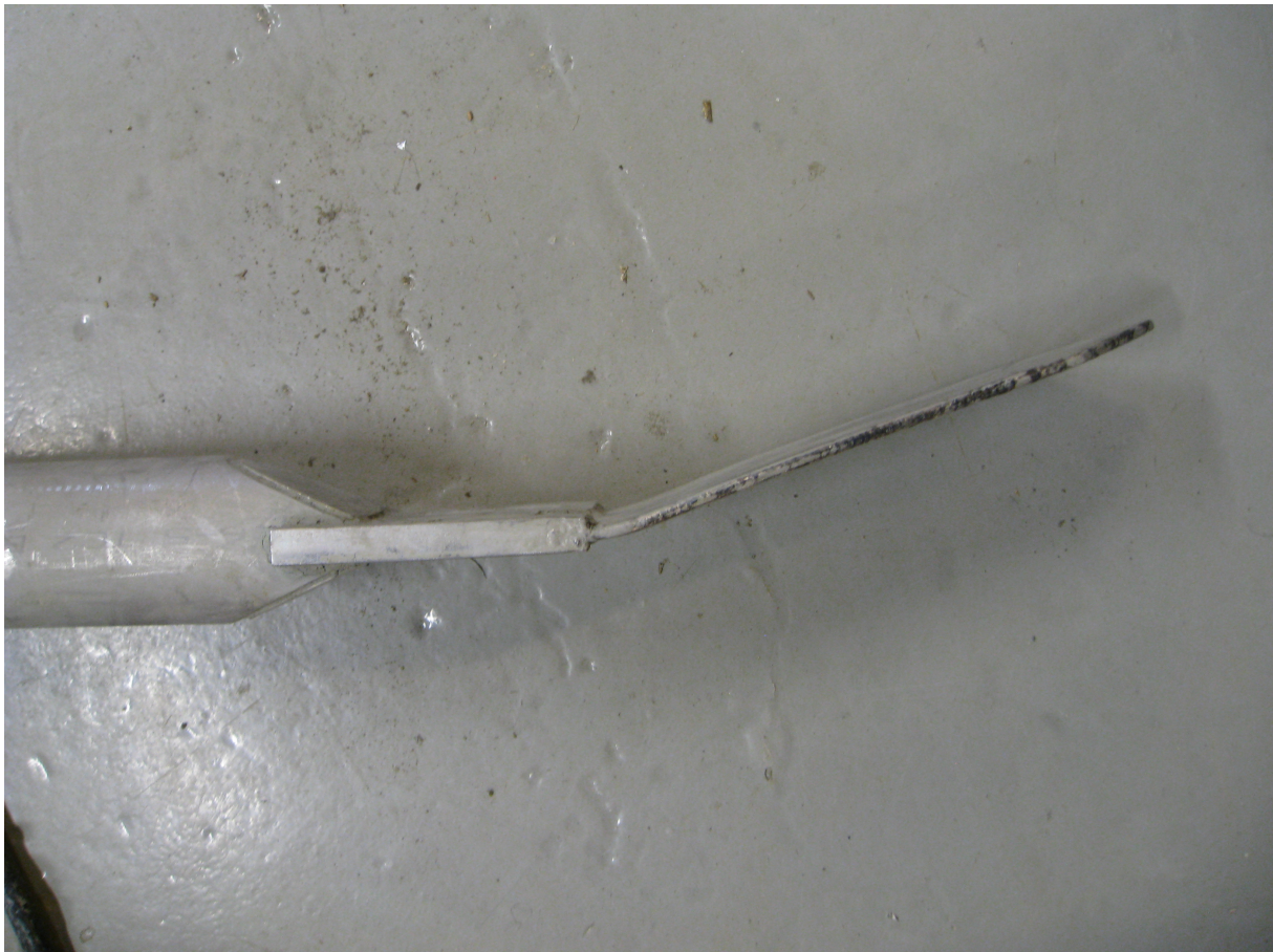
(b) Second cell damaged during penetration to 8 m. Earth pressure sensor EE24692.
