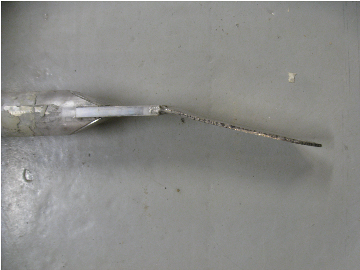
Figure 3.5: Cell damaged during penetration to 10 m. Earth pressure sensor EE24712.
