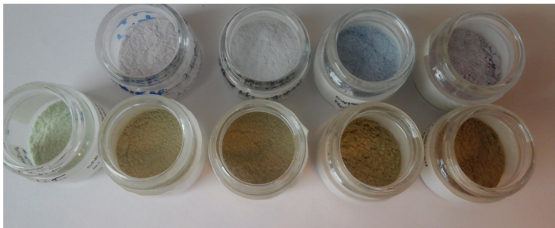
Picture 1: On top: The prepared 5wt% Ni-Co hydrotalcite precursors, from left to right: 3.5Ni-1.5Co HT, 2.5Ni-2.5Co HT, 1.5Ni-3.5Co HT and 5Co HT. To the bottom: the mixed oxide catalysts derived from these hydrotalcite precursors after the treatment at 600°C for 6h. From left to right: 5Ni, 3.5Ni-1.5Co, 2.5Ni-2.5Co, 1.5Ni-3.5Co and 5Co mixed oxides.
