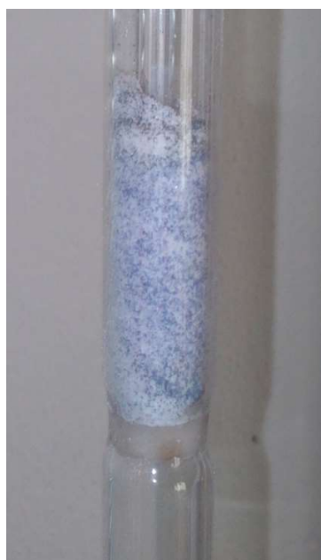
Picture 2: 12wt%Co mixed oxide catalyst diluted in \text{Al}_2\text{O}_3 after methane combustion.
