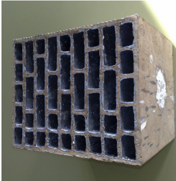
Figure 7 Hollow brick with low-e coating on the inner surfaces, schematic drawing (top) and photo (bottom) (Principi and Fioretti [61]).
