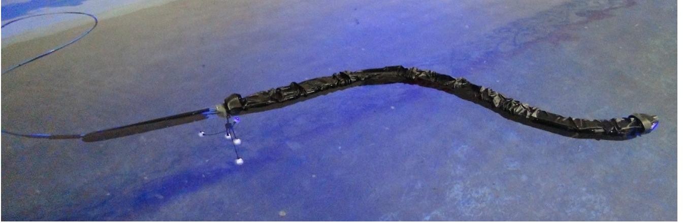
(b) Underwater snake robot Mamba with passive caudal fin attached at the last module of the robot
