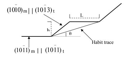
Fig. 3 Schematic diagram showing the deviation angle between the twin boundary trace and the twin plane caused by the step-terrace structure of the faceted twinning boundary.
