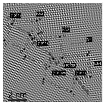
Fig. 2 Inverse fast Fourier transform (IFFT) image of the boxed area shown in Fig. 1c. Burgers circuits are drawn around three steps. . In the figure, the steps are parallel to
