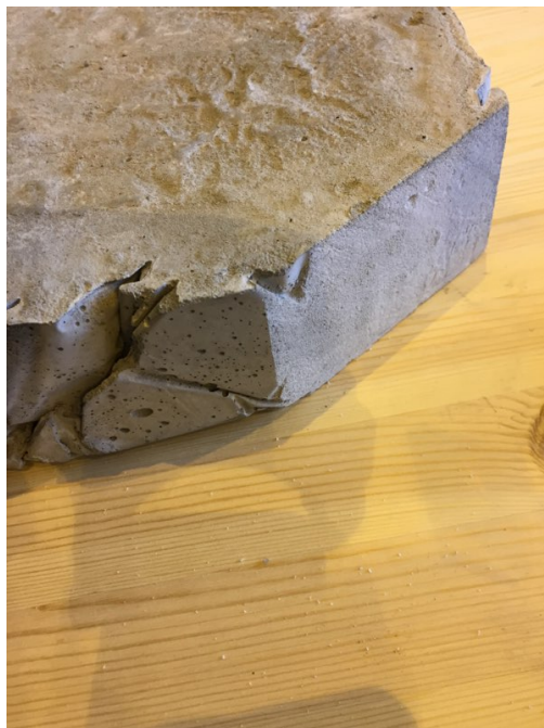
Figure D.2.3: Picture of the finished product. Some of the rock samples were sawed, so it could be easier to study the distribution of the sand and the cement within the rock samples.
