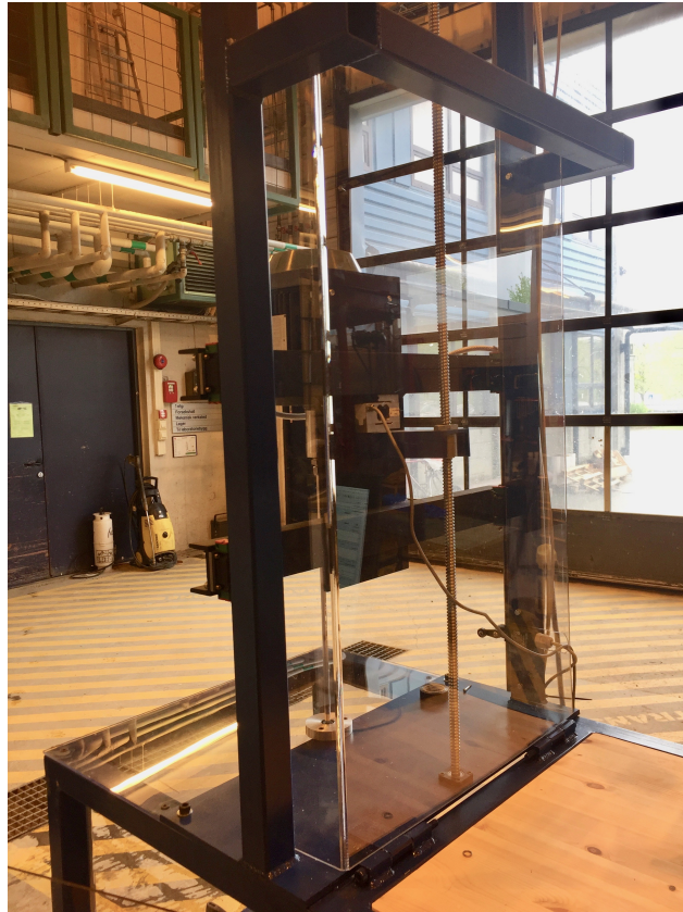
Figure 2.6: Plexiglass mounted to the derrick, isolating high pressure zones from working personnel
