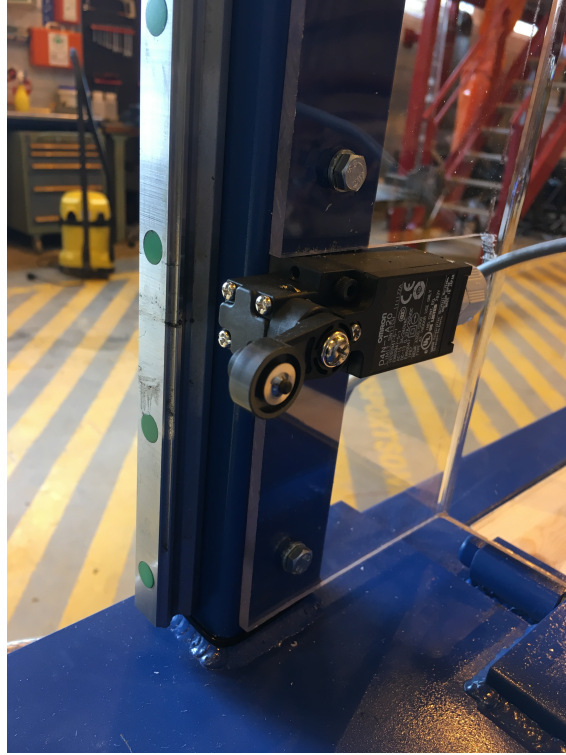
Figure 2.4: Stopping mechanism on the extremities of the rail
