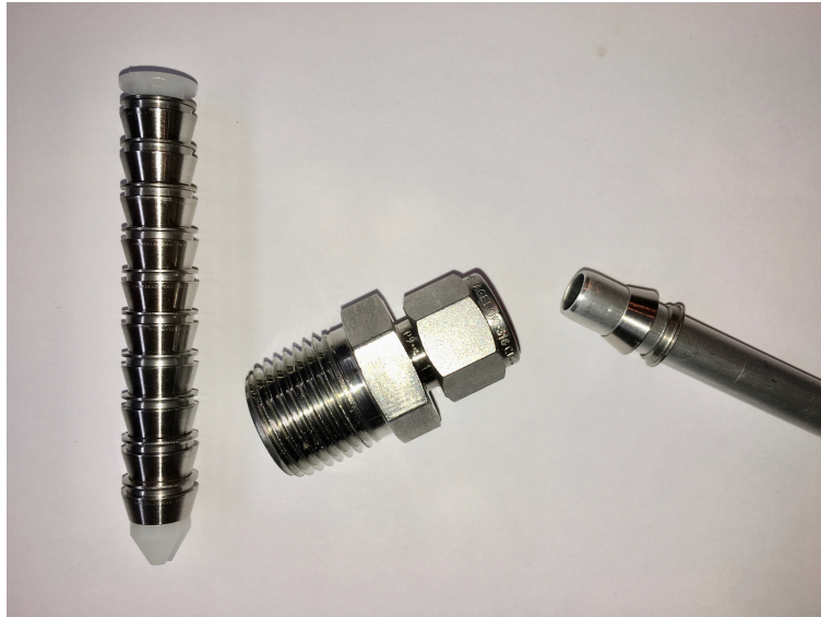
Figure 3.1.12: Hydraulic connections used as tool joints between BHA and pipe, and between pipe and swivel
