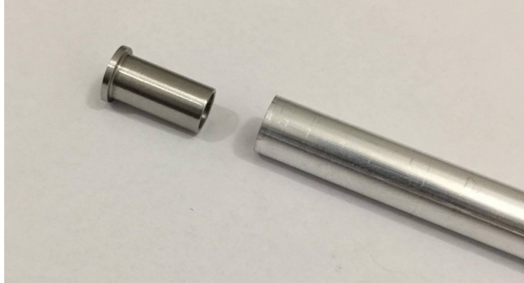
Figure 8.4.1: Steel cylinder placed inside the pipe at connection point to increase strength
