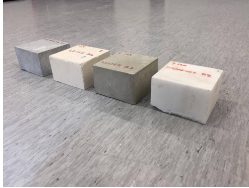
Figure D.2.6: Picture of the rock samples provided by SINTEF. Marble in the right, two different types of sandstones in the middle and and dolomite in the left.
