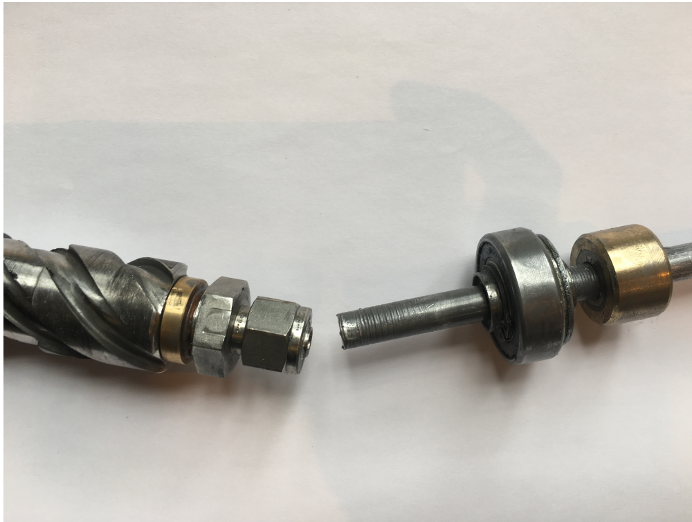
Figure 7.3.2: The first twist-off
