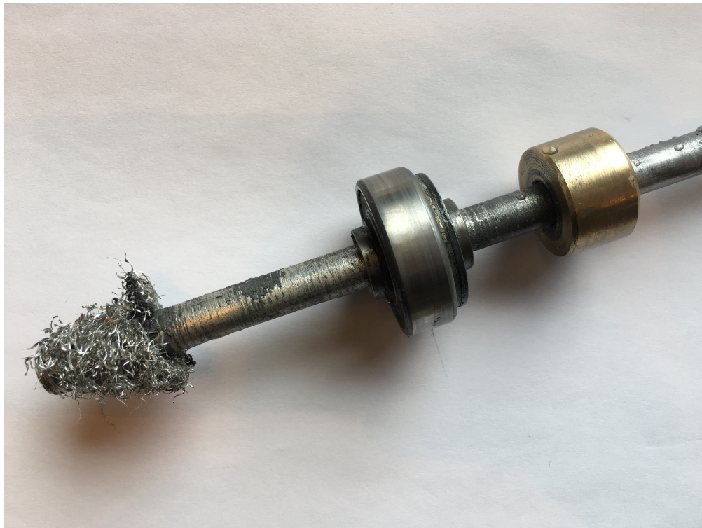
Figure 7.3.3: The second twist off
