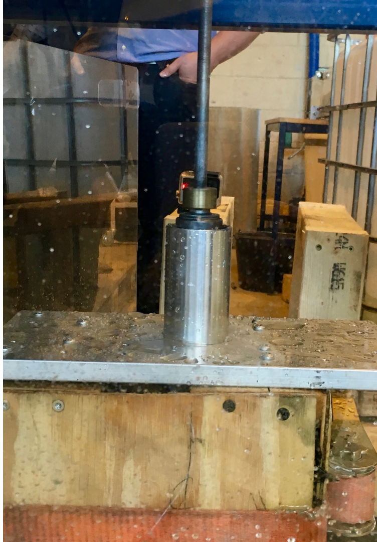
Figure 3.1.17: Landing of the surface stabilizer inside the riser. Picture from on-site test day.
