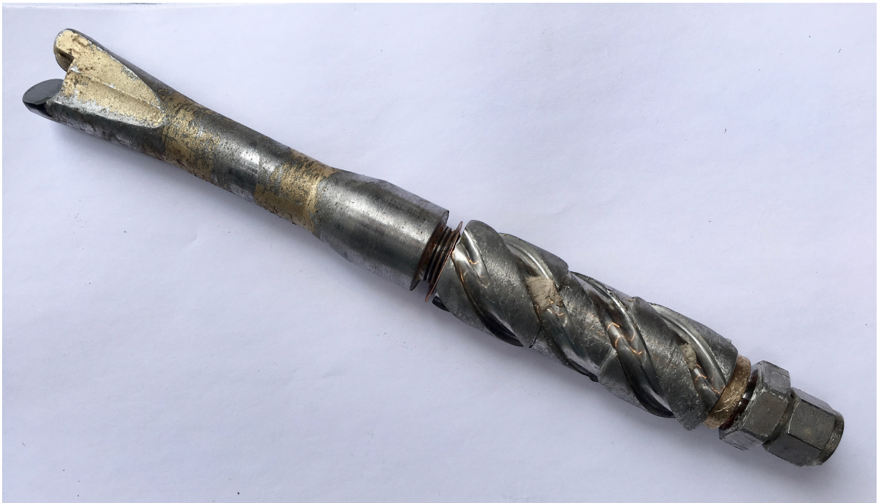
(b) Picture of the bit and BHA used on competition day
