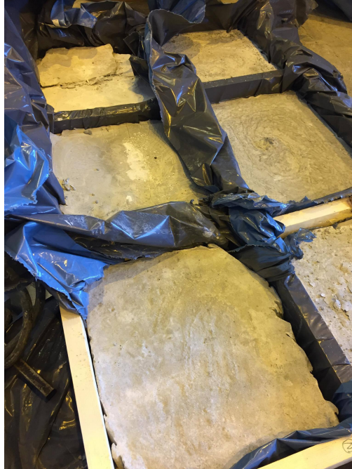
Figure D.2.2: Picture of a homemade "sandstone" in the making. The mixture of sand, water and cement is poured into the forms and is ready to solidify.
