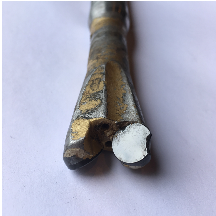
Figure 7.4.2: Wear on the bit cutters and bit body
