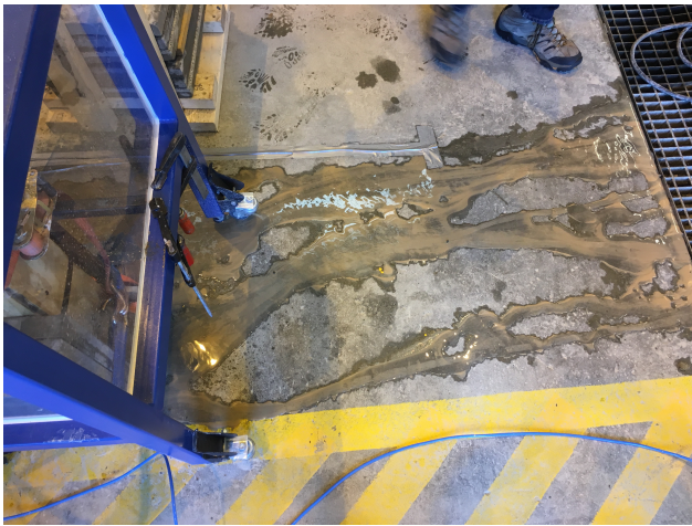
(a) Return flow from annulus indicating sandstone was being drilled
