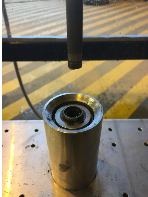
Figure 5.3.10: Twist-off at the connection between the BHA and the drill string when drilling asphalt
