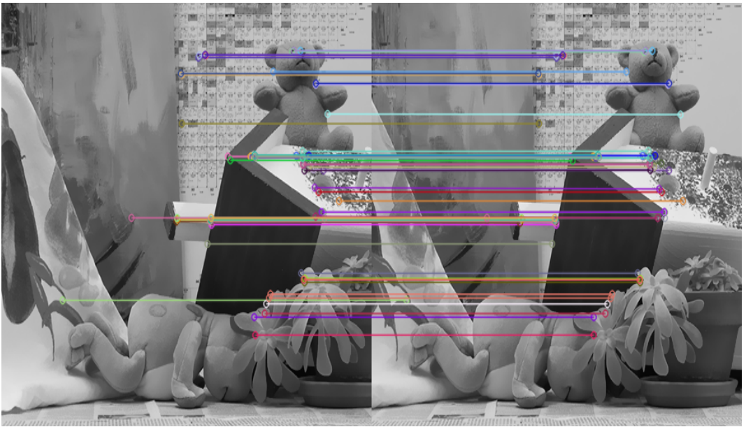
Figure 4.17 Point matches between a perfectly rectified image pair.
