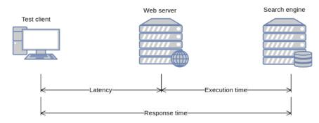
Figure 5.3: Overview of the different measurements used when evaluating the implementation.
