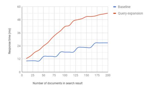
Figure 5.5: Response times using different result sizes with cache prewarming.
