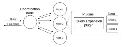
Figure 4.3: Architecture for the implemented Elasticsearch plugin. The figure is an example of a cluster setup with a view inside one of the nodes in the cluster.
