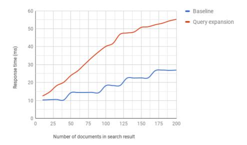
Figure 5.6: Response times using different result sizes without cache prewarming
