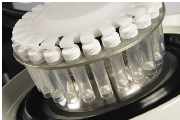
Figure 1.2: The beads-based homogeniser used in this project, a Precellys 24 tissue homogeniser. Cryo tubes containing beads are seen loaded into homogeniser. [13].
