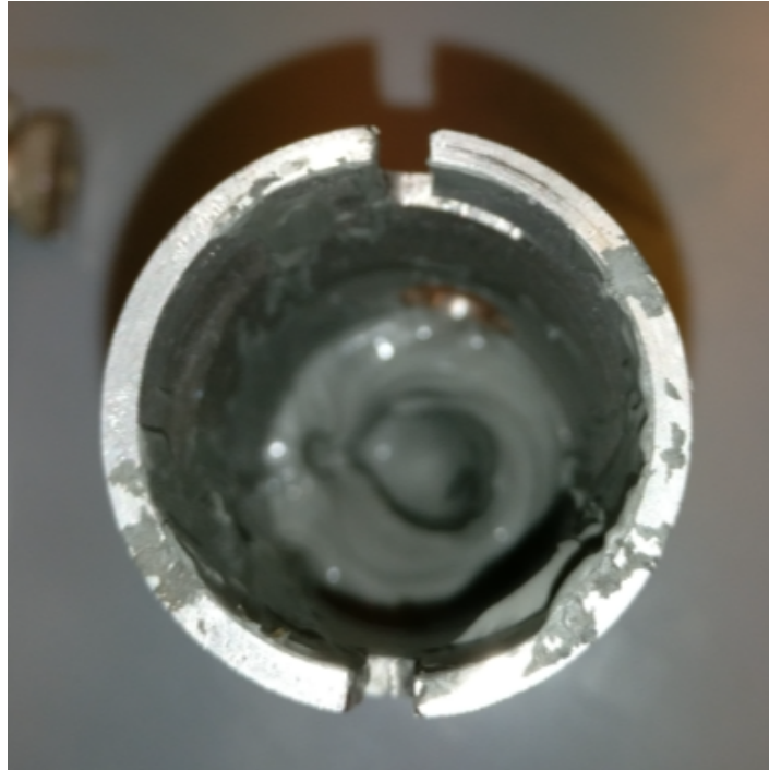
Figure 5.16: Observed slippage between spindle and clay with high remoulded shear strength. Hole remains in clay after the spindle has been removed.
