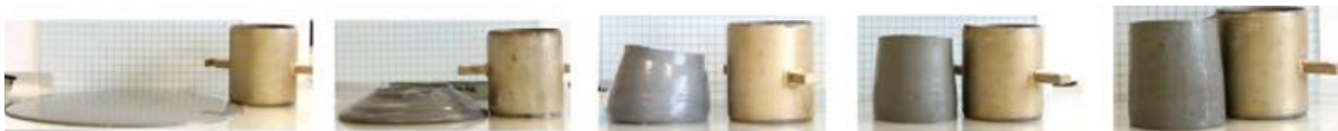
Figure 2.15: Slump and spread observed for remoulded Byneset clay, Norway. Quickness tests performed at c_{ur} = 0.1 kPa, 0.2 kPa, 0.5 kPa, 1.1 kPa and 2.0 kPa. From Thakur and Degago (2014)
