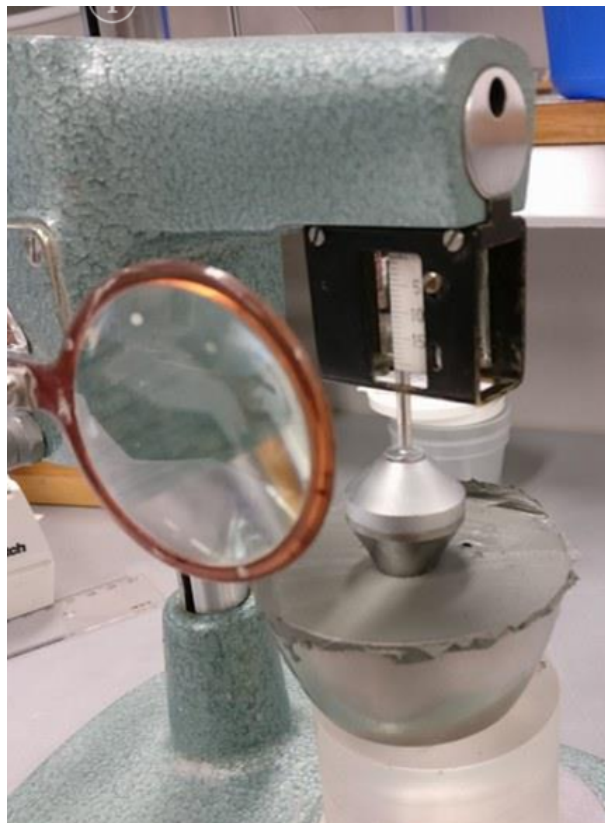
Figure 2.5: Fall-cone test used to determine the remoulded shear strength of clays. Measured penetration used along with calibrated tables to provide point-specific shear strength.
