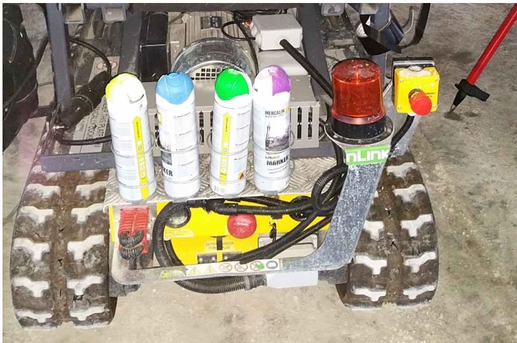
FIGURE 4.27 EMERGENCY STOP AND WARNING LIGHT (OLE ROSENLUND, 2017)
