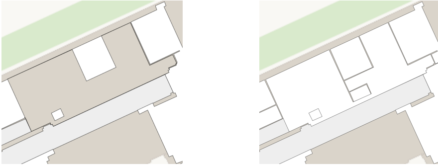
Figure 7.6: Left: Undesirable merging result. Right: Rooms before merging
