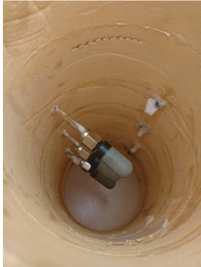
Figure 3.4: Filter stones inside the freezing cell
