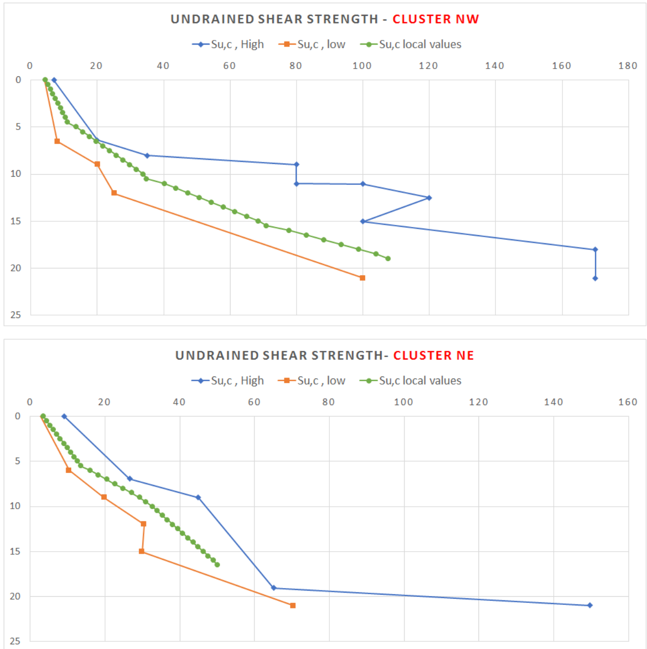
Figure B.1: Recommended undrained shear strength for NW and NE cluster (NGI, 2007).
