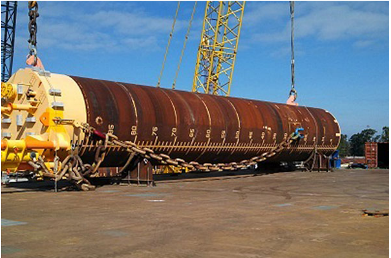
Figure 2.4: Illustration of suction anchor with chain attached to a pad-eye (Source: Technology).
