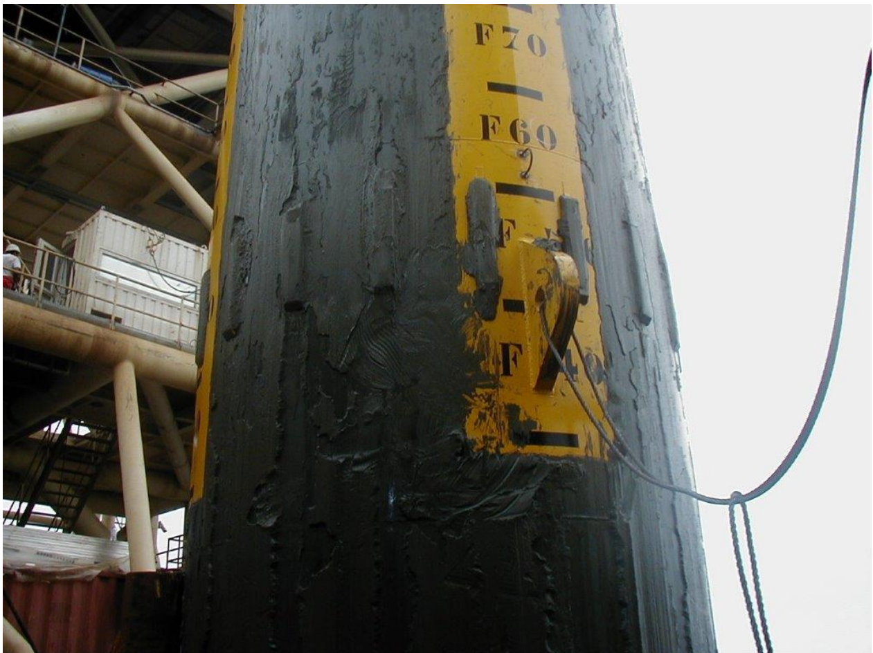
Figure 3.3: Thick layer of clay sticking to the sides of an suction anchor after being pulled out at the Girasoll oil field. The picture also illustrates how soil fail in the interface between the anchor and clay for where the anchor was painted. Source: Gisle Håland.
