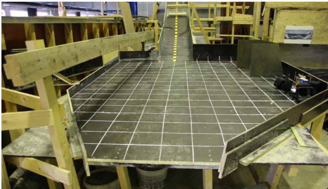
Figure 13. The runout table of the debris flow model after it was repainted. The table is 360 cm long and the grid is 20 x 20 cm (Laache, 2016).
