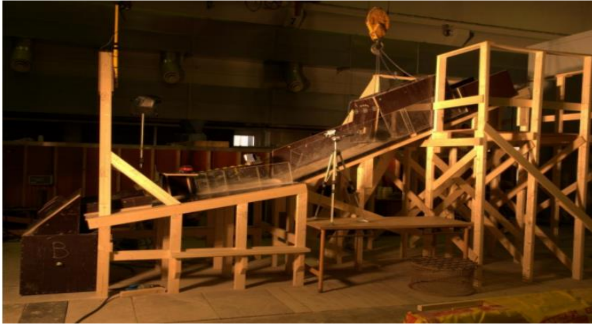
Figure 12 The debris flow model in 2009 when it was used to investigate the effect of channeling debris flows under a bridge by using deflection structures (Hiller & Jenssen, 2009)
