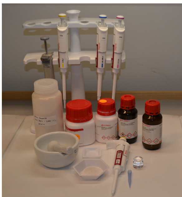
Figure 3: Set up used for impregnation of dolomite
