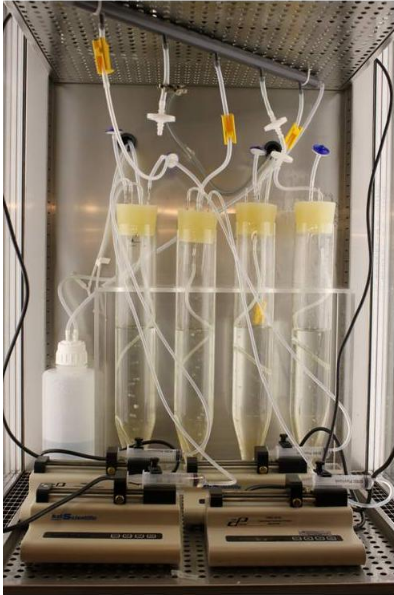
Figure 12: Setup for continuous feed solution delivery.
