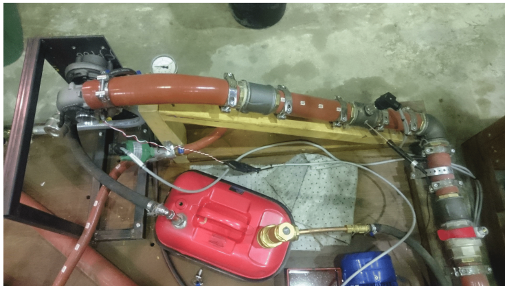
Figure 4.1: The laboratory layout of the compressor model simulation. The turbocharger is located in the upper left corner and throttle valve in the lower right corner. The red tank in the center is the oil lubrication-loop reservoir
