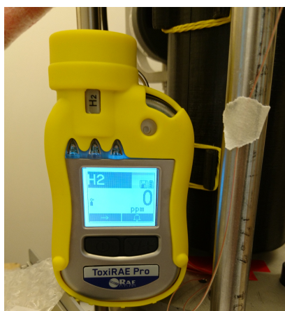
Figure B.1: ToxiRAE Pro single gas detector set to detect hydrogen.
