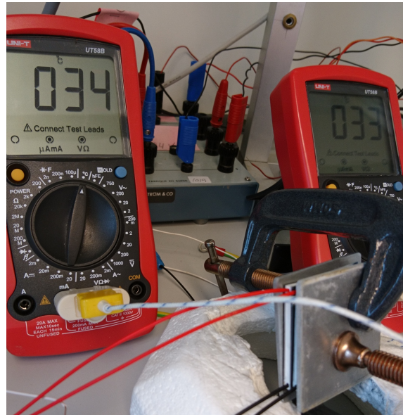
Figure C.1: Two clamps clamp the two peltier modules together as well as a thermocouple on each outer side.
