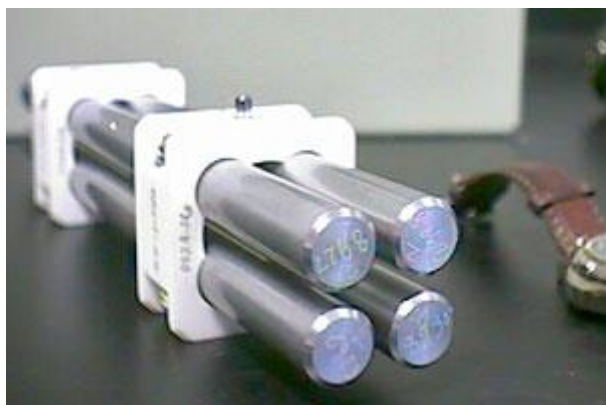
Figure 1-9: The 4 cylindrical rods of a quadrupole mass analyzer (Worley and Kvech 1999).
