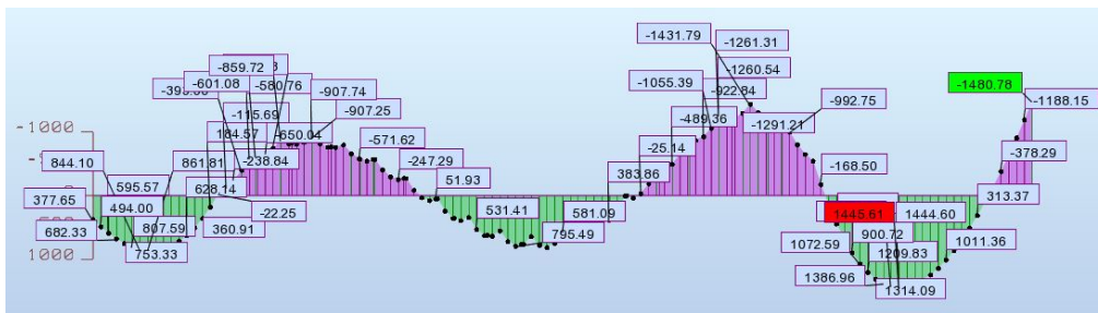
Figure 5.4: Diagram of M_y for the arch using Robot. Loading: self-weight
