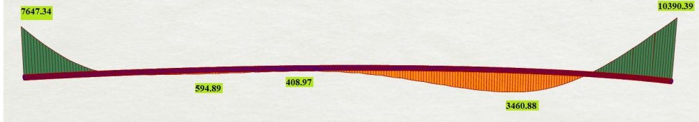
Figure 5.12: Diagram of M_y for the inner tubular beam using Karamba. Loading: 16(C).
