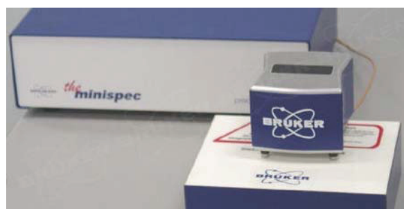
Figure 25: Low field unilateral Bruker Profiler NMR surface scanner used in Paper V.
