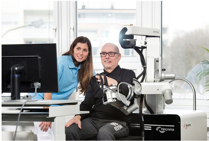
Figure 1.1: Example of robotic rehabilitation with stroke patients using an exoskeleton device called ArmeoPower. Figure taken from [16].
