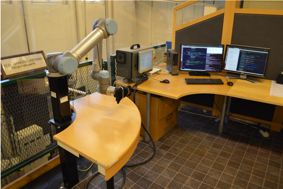
Figure 3.11: Completed system setup. The UR5 robot manipulator is mounted on the pedestal. Prototype 1.1 is mounted to the end-effector with an illustrative glove attached. In the background, the Controller Box with the teach pendant attached on the front together with a PoE switch and an external computer. The F/T Net Box is hidden from view behind the tabletop.
