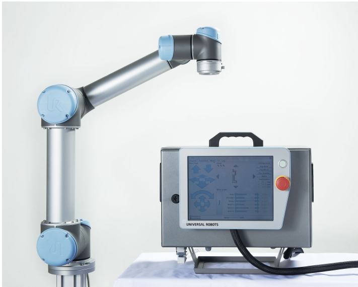
Figure 3.1: System overview of the UR5 robot from Universal Robots. The system consists of three main components. The six-axis robot manipulator on the left, the Controller Box centered on the table and the teach pendant attached to the front of the Controller Box. Figure taken from [30].
