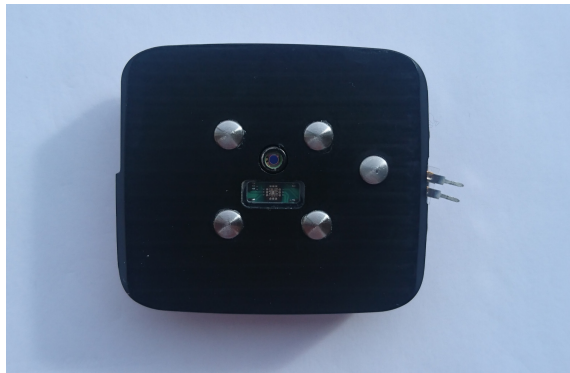
Figure 2.6: Impedance electrode modified to be the actuator
