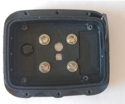
(b) Inside of Prototype II bottom casing with actuator visible to the left
