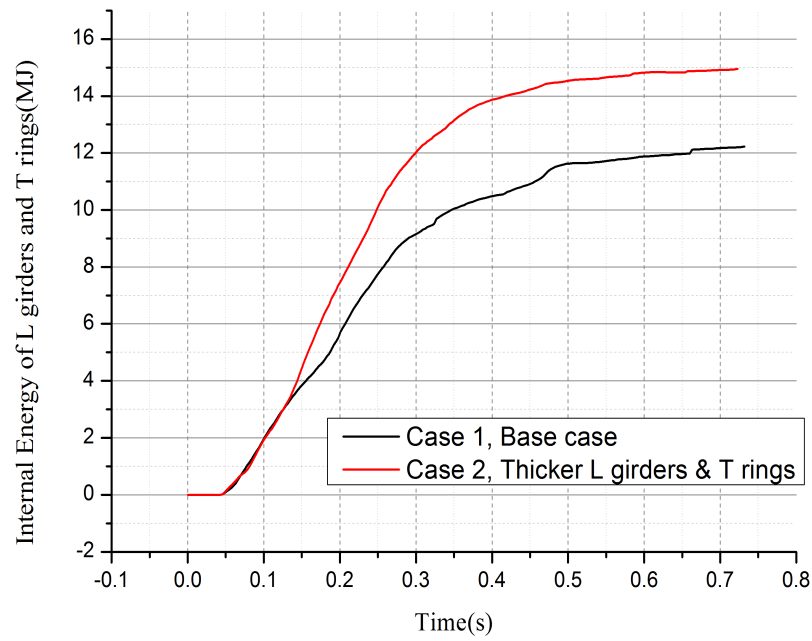
Figure 3.21: The internal energy of the L profile girders and T profile rings in case 1 and case 2
