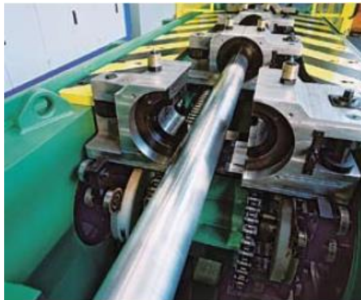
Figure 11: Split clam caterpillar capstan [19]
