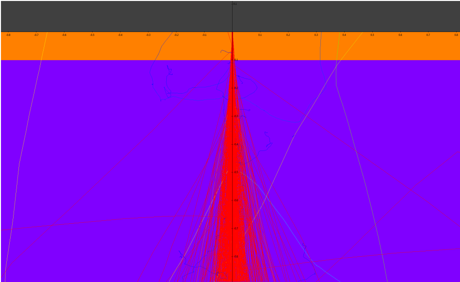
Figure B.3: Detailed view of the electron trajectories in the substrate boundary.
