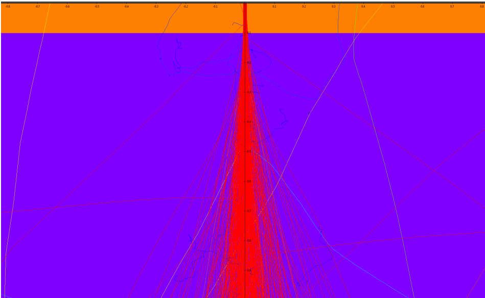
Figure B.11: Detailed view of the electron trajectories in the substrate boundary.
