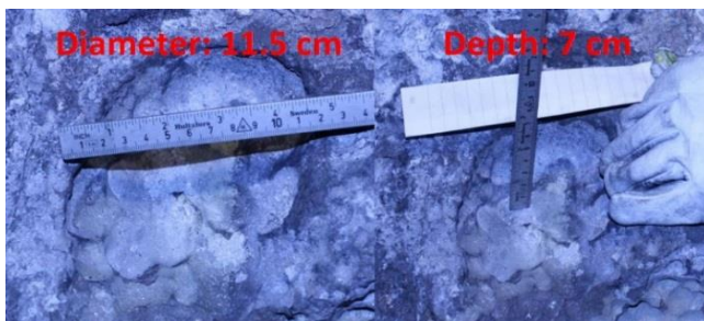
Figure 5. A pothole showing the smaller pittings that joined to form it. The diameter and depth are also shown.
