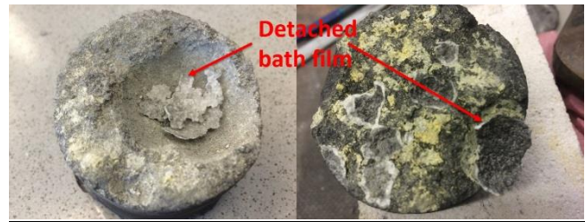
Figure 6. Autopsy samples showing the detached thin bath film. The yellow colour at the surface is aluminium carbide. Aluminium carbide could be observed under the detached thin bath layer on the sample to the left.
