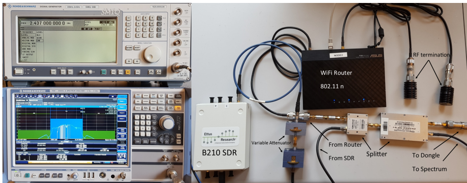
Figure 5.10: Pictures of the jamming experiment. Spectrum analyzer and signal generator are depicted on the left.
