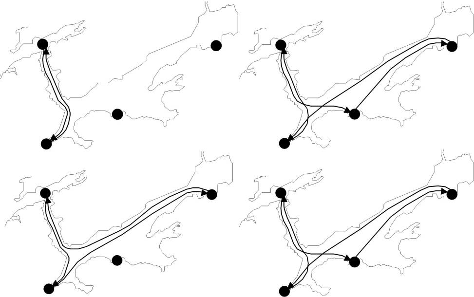
Figure 13: Illustration of routes generated from step 2 of optimization model. Expectation values of transportation demand and port opening hours from 07.00 to 15.00.
