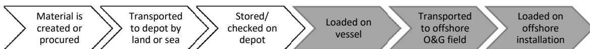
Figure 2: Flow of material through upstream offshore supply chain from production/procurement to offshore installations. The grey stages are done by PSV's.
