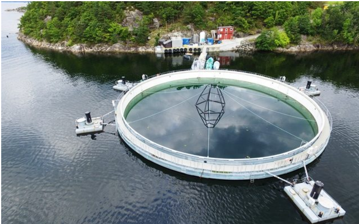
Figure 1.2: Neptun, a prototype semi-closed system from Marine Harvest and Aquafarm Equipments. The size and design of this system is used further on in this study. This type of system are so far being operated much closer to shore than is the case for traditional open net pen systems. (Retrieved 16.02.2017, from: http://kyst.no/nyheter/satt-ut-smolt-i-lukka-merd/ )
