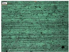
**Figure 4.2** Optical micrograph of the AA6082-T6 base metal microstructure parallel to the plate rolling direction at high magnification (20x). (The scale bar in the upper left corner is  $50 \ \mu m$ ).
