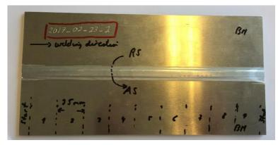
*Figure 3.2 Photograph of the butt welded plates received from HyBond AS. Shown is also the welding/rolling direction and the retreating/advancing side.*
