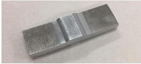
**Figure 3.4** Photograph of the specimen used for micrographic examination and hardness testing.
