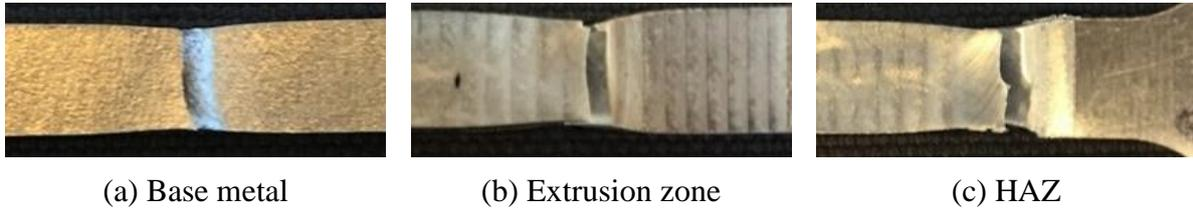
**Figure 4.11** Examples of macro-images of tested tensile specimens showing the fracture point in each of the zones.
