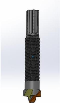
*Figure 2.31 Solid Works drawing of the conical pin used for HYB butt joining of plates. (Ø. Grong, Personal Communication, 2017).*
