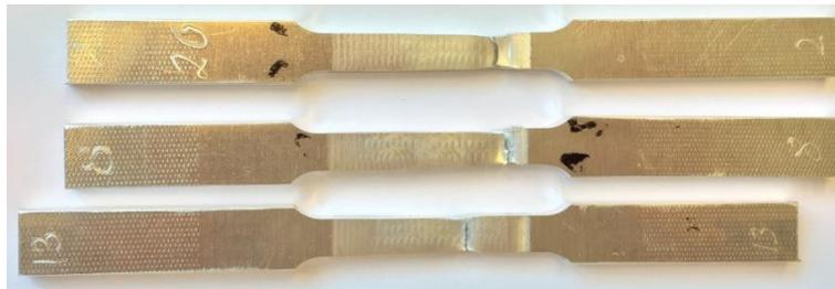
**Figure A 5** Measured stress-strain curves for the HAZ. Included are also macro-images of the tensile specimens subsequent to testing. (Specimen 8 is presented in the report).
