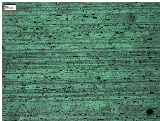
**Figure 4.2** Optical micrograph of the AA6082-T6 base metal microstructure parallel to the plate rolling direction at high magnification (20x). (The scale bar in the upper left corner is 50 μm).
