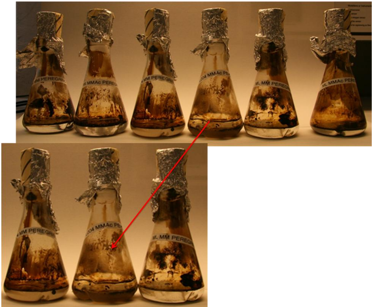
Figure 29. Peregrino – after incubating for seven days at 60°C Visual growth is observed in sample L004 MM and L004 MMac (enlarged).
