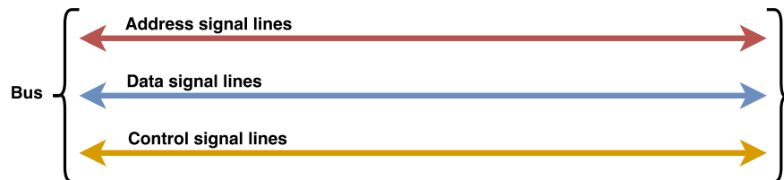
Figure 2.4: An example of bidirectional bus lines. Adapted from Source: [27]
